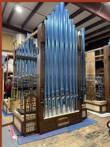
Blue film protects the façade pipes as they are set up in the shop.
