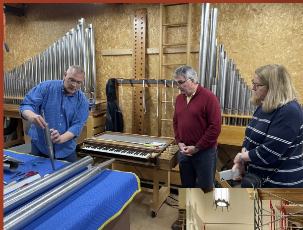
The lowest pipes of the 32' Contrebasse were the first to be assembled.
