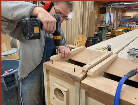
The lowest pipes of the 32' Contrebasse were the first to be assembled.
